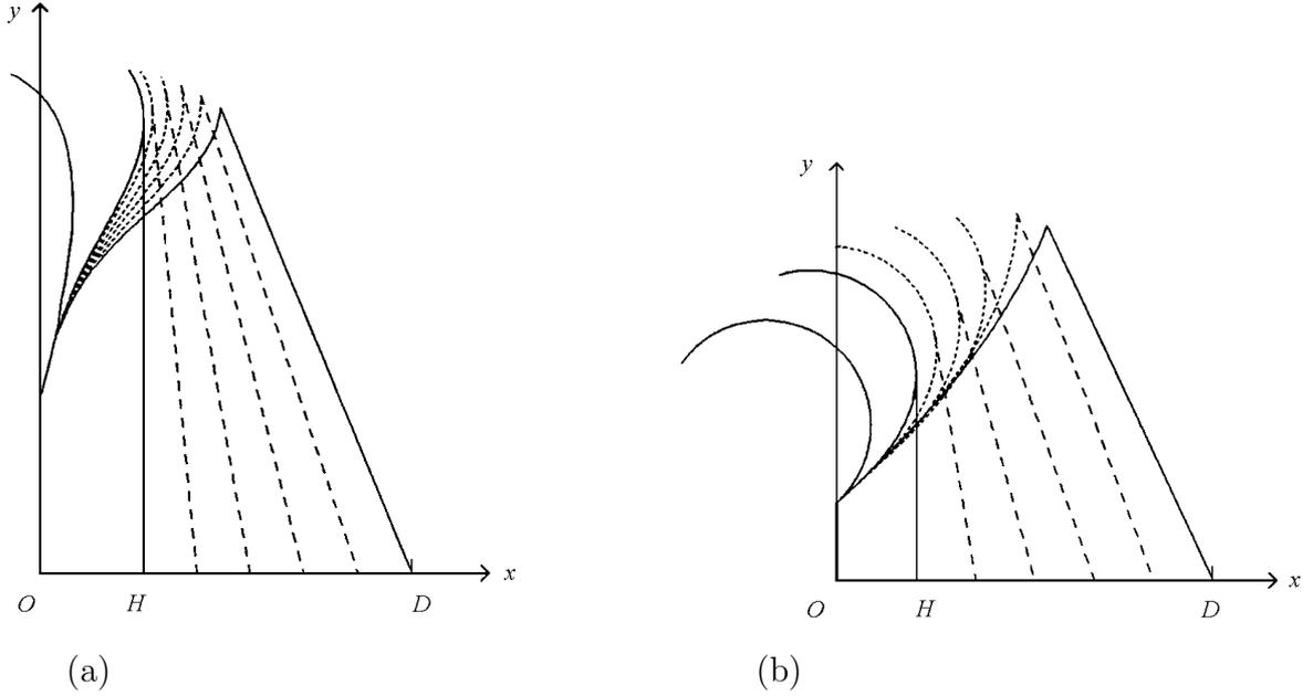
Figure 8: (a) Dimensionless deformations of the  $B_1$  bow. (b) Dimensionless force-draw curve of the  $B_2$  bow.
