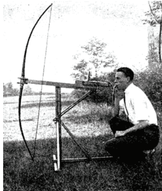
The author with a shooting machine which he designed for use in testing arrows. This machine was used in conjunction with a chronograph for measuring the velocity and acceleration of arrows. It is equipped with pneumatic release.
